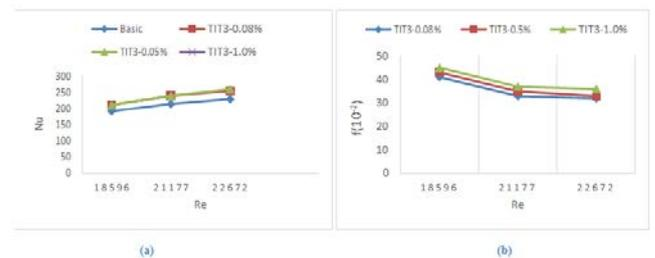
Figure (a) Effect of Al2O3/EG nano fluid volume concentration on Nusselt no. of nano fluid with tube insert (b) experimental friction factor of EG and different volume concentrations of Al2O3 nano fluid with tube inserts.
