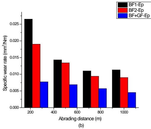
Figure 3: (a) volume loss V/s abrading distance and (b) Specific wear rate V/s abrading distance for different samples at 23N
