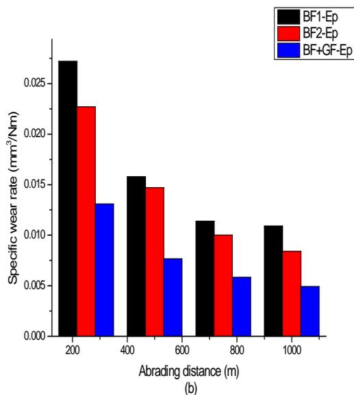
Figure 4: (a) volume loss V/s abrading distance and (b) Specific wear rate V/s abrading distance for different samples at 36N
