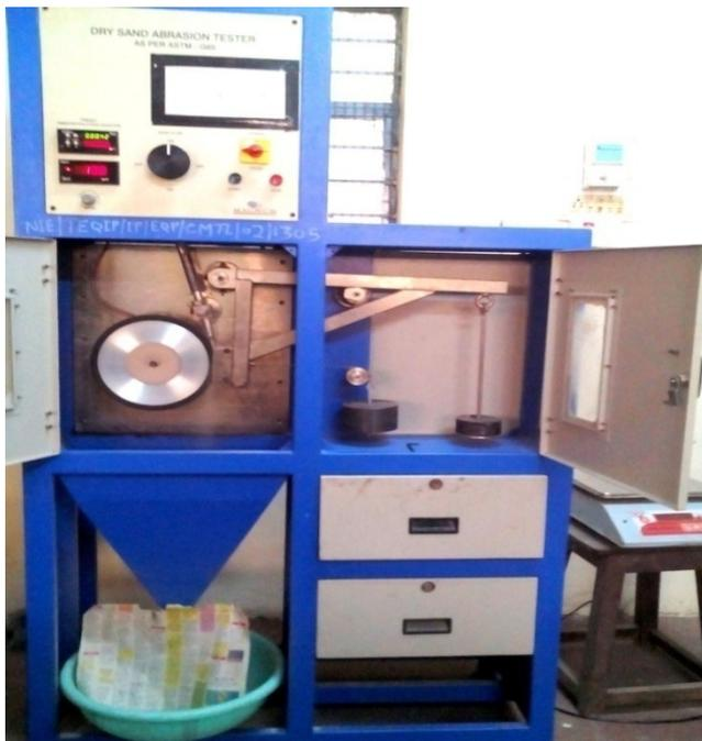
Figure 2: Three body abrasive wear setup
