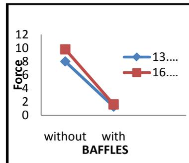
Chart 1 – Comparison of water impact force on container walls due to slosh during braking of vehicle.
