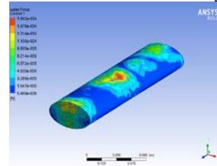
Fig 9 Water impact force acting on the container walls with baffle at vehicle velocity of 16.88 m/s
