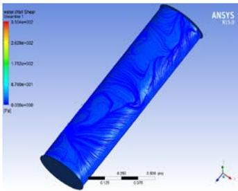
Fig 5 Wall shear & Streamline without baffle at 16.88 m/s
