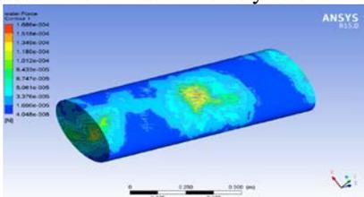
Fig 7 Water impact force acting on the container walls without baffle at vehicle velocity of 16.88 m/s
