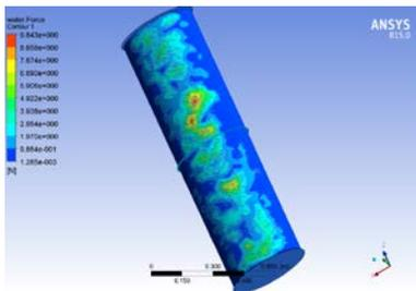
Fig 6 Water impact force acting on the container walls without baffle at vehicle velocity of 13.88 m/s
