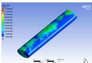
Fig 8 Water impact force acting on the container walls with baffle at vehicle velocity of 13.66 m/s
