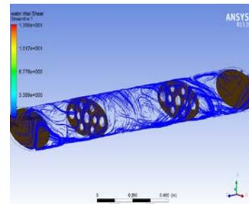
Fig 10 Velocity Streamline of Water slosh inside the container with baffles at 16.88 m/s
