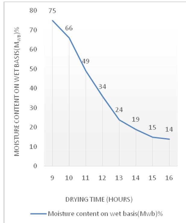
Fig.3. Drying Time vs Moisture content
