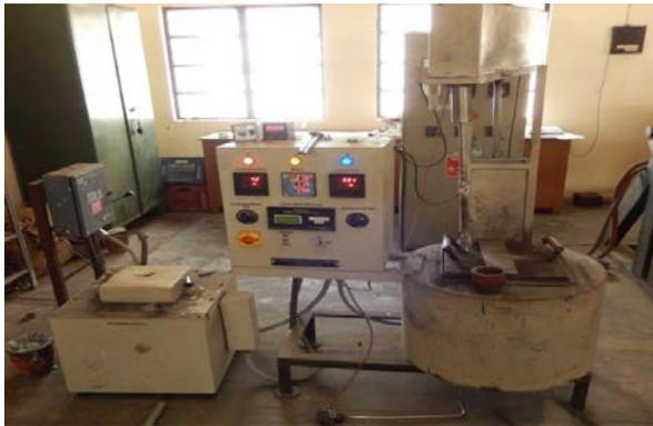
Fig.1. Stir casting setup
