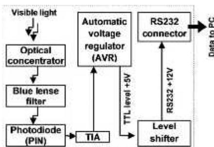
the practical down-conversion technique is direct detection (DD), in which a PIN photodiode sensor
