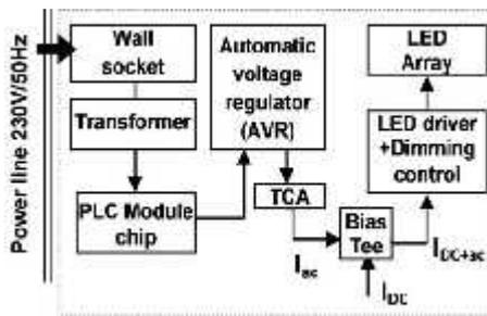
Figure . Block diagram of PLC receiver and VLC transmitter
