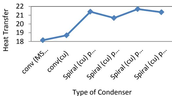
Fig.5.4. Heat Transfer vs Type of Condensor
