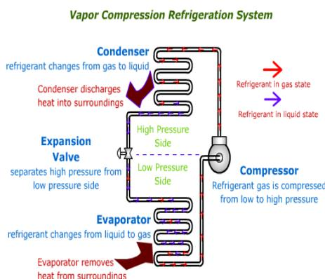
Fig. 1.1. Vapour compression refrigeration system
