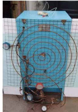
Fig.3.5 Spiral with Pitch(50.8mm)
