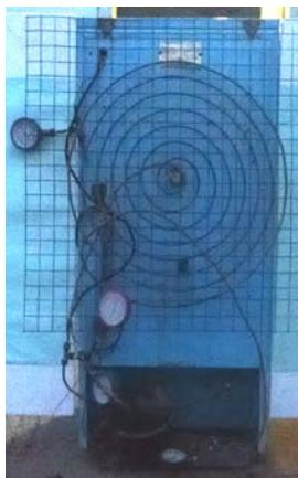
Fig.3.3 Spiral with Pitch(38.1mm)
