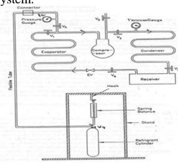
Fig.3.7. charging of refrigeration system
