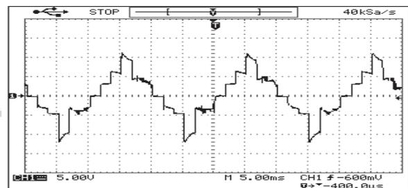
Fig.11. Output current of seven level asymmetry diode clamped multilevel inverter
