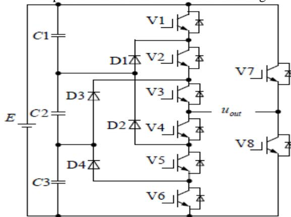
Fig.1. Schematic diagram of asymmetry diode clamped seven-level inverter
