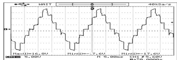
Fig.10. Output voltage of seven level asymmetry diode clamped multilevel inverter
