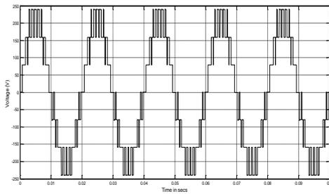
Fig.6. Output voltage waveform for asymmetry diode clamped Multilevel Inverter
