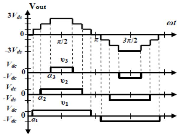
Fig.2: Output waveform of seven level Asymmetric diode clamped multilevel inverter
