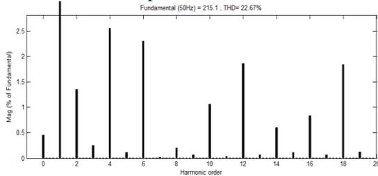
Fig.7. Harmonic spectrum of asymmetry diode clamped multi level inverter
