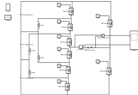
Fig.4. Simulation of asymmetry diode clamped multilevel inverter
