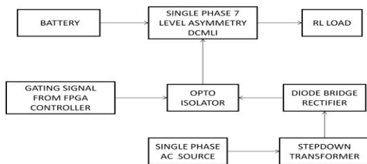
Fig.8. Block diagram of asymmetry diode clamped multilevel inverter
