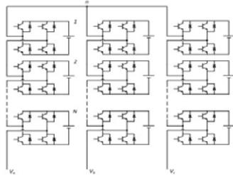
Figure 3.2 - Topology of Cascaded H-Bridge Inverter
