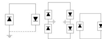
Figure 2.1 - HVDC system configurations. (a) Mono polar. (b) Bipolar. (c) Back-to-back
