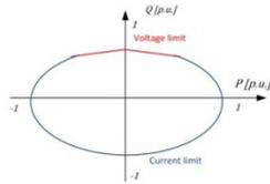
Figure 2.2 - Active-reactive locus diagram of VSC-HVDC transmission
