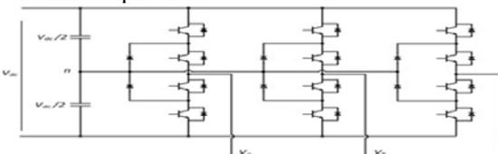
Figure 3.1 - Topology of three level NPC converter
