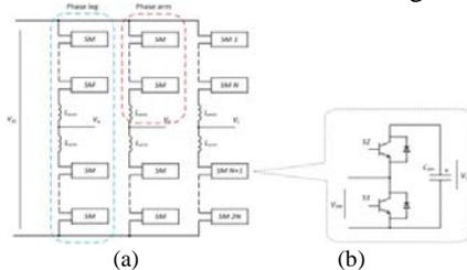
Figure 3.3 - (a) Topology of three-phase MMC (b) Half-bridge sub-module
