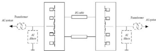
Figure 2.4 - MMC-HVDC system configuration
