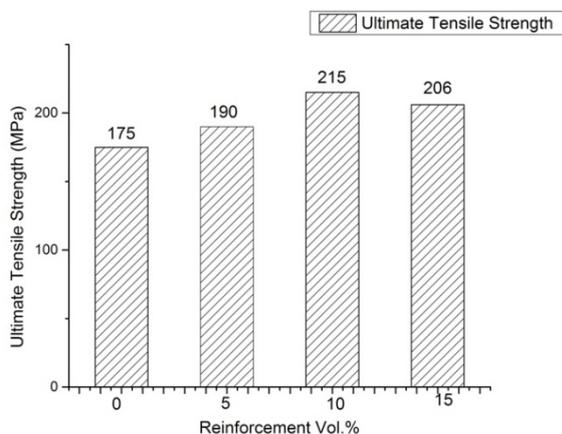
Figure 6: Tensile Strength of Red mud reinforced Aluminium 7075 composite
