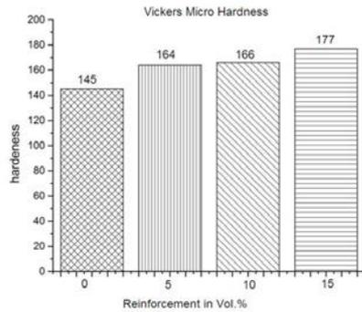
Figure 4: Vickers Micro Hardness values of Red mud reinforced Aluminium 7075 composite.
