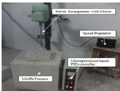
Fig. 1. Stir Casting Setup
