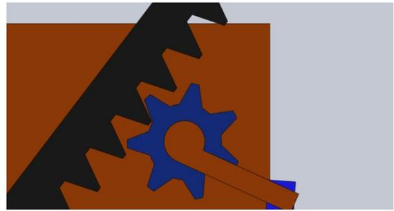
Fig 5 GEAR AND PINION MECHANISM
