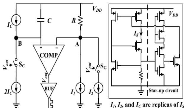
Fig. 1 Schematic illustration of the proposed DT technique and bias circuits.
