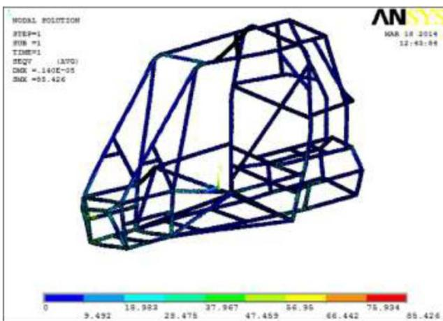
Fig:10.front impact analysis 8500N at front FOS=2.686
