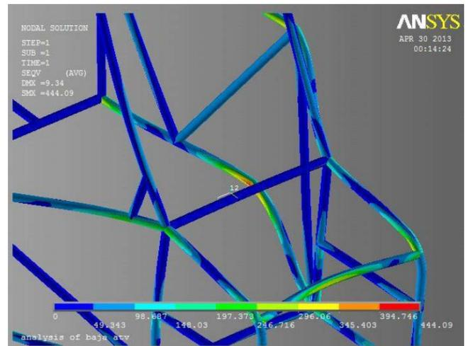
Fig:06. Region of high stress concentration in Fig :04
