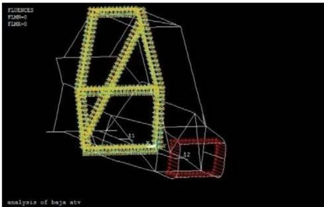
Fig: 03. Loading points and impact points
