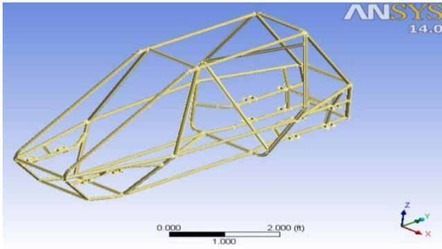
Fig:12 Isometric view of roll cage
