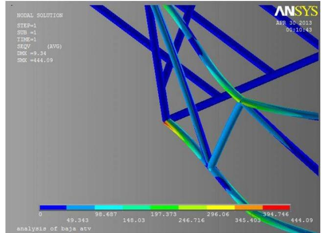
Fig:05. Region of high stress concentration in Fig :04
