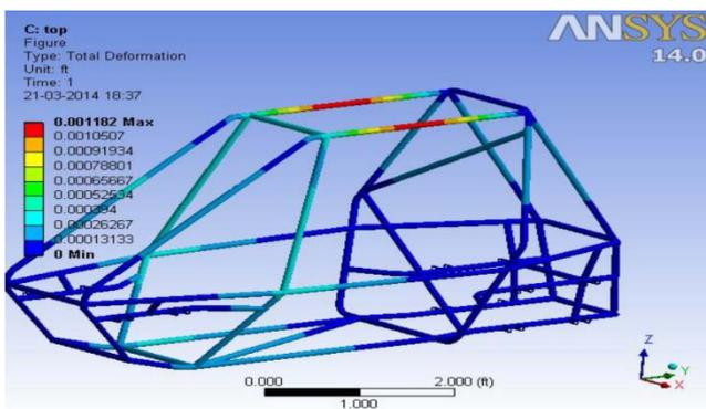
Fig:14. Deformation due to roll over.
