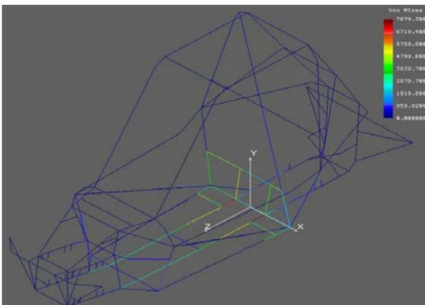
Figure 02: second static analysis, with revised frame design for optimum stress distribution
