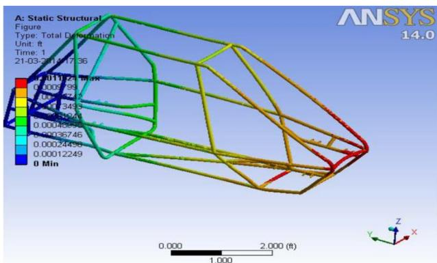
Fig:13 .Deformation due to front impact load
