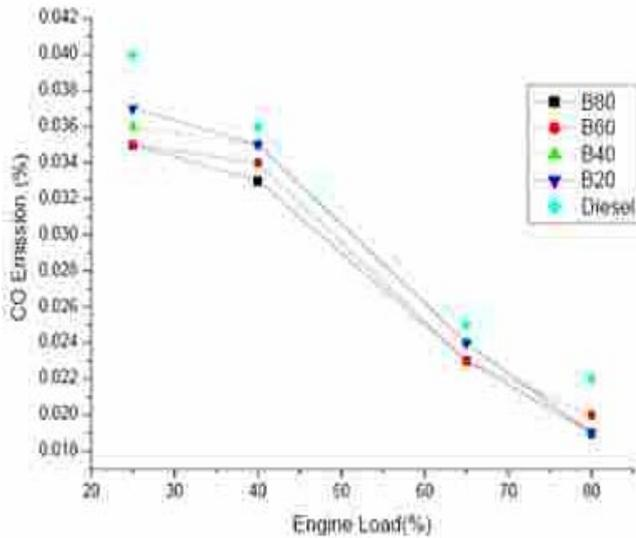
Fig.8 Carbon monoxide Vs Load
