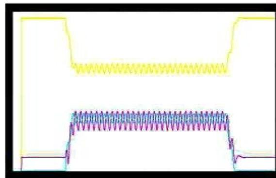
Figure (f):- When 2L-G Fault Is Created, Three Phase Sequence
