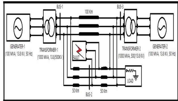
Figure (a) :- Model For Transmission Line Fault Analysis.
