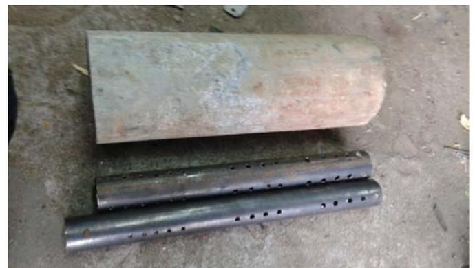
fig2: Tubes drilled with holes of different diameter
