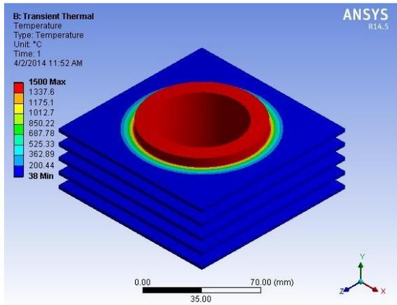
Fig. Temperature distribution for 2.5 mm thick rectangular fin
