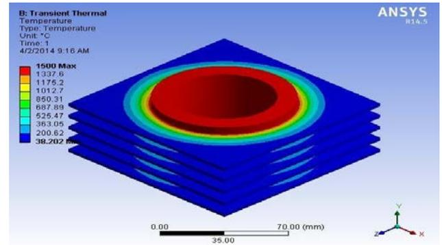
Fig. Temperature distribution for 3 mm thick rectangular fin
