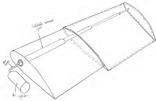
Figure 2: Pneumatics Mechanism
