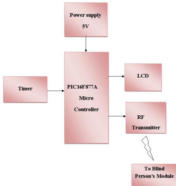
Fig. 2. Block Diagram of Traffic Module
