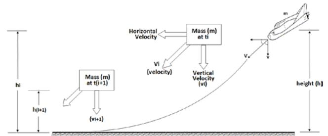
Fig. 3. Determination of landing path
