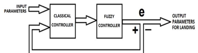
Fig.1. Basic idea of fuzzy logic integration for landing application
