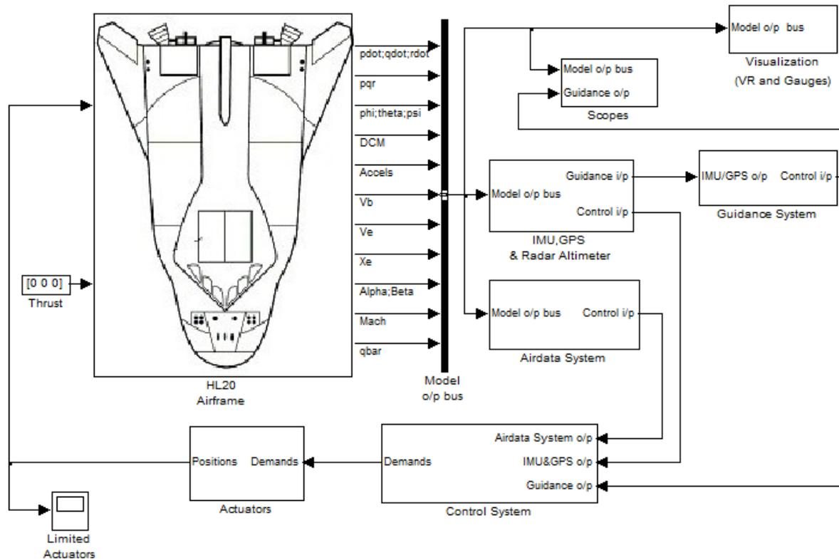
Fig. 5. Landing controller design of NASA's HL 20. (source: mathworks [10])
