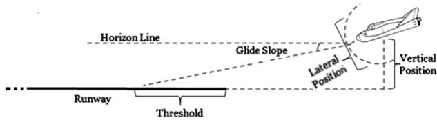
Fig. 2. Desired final approach path
