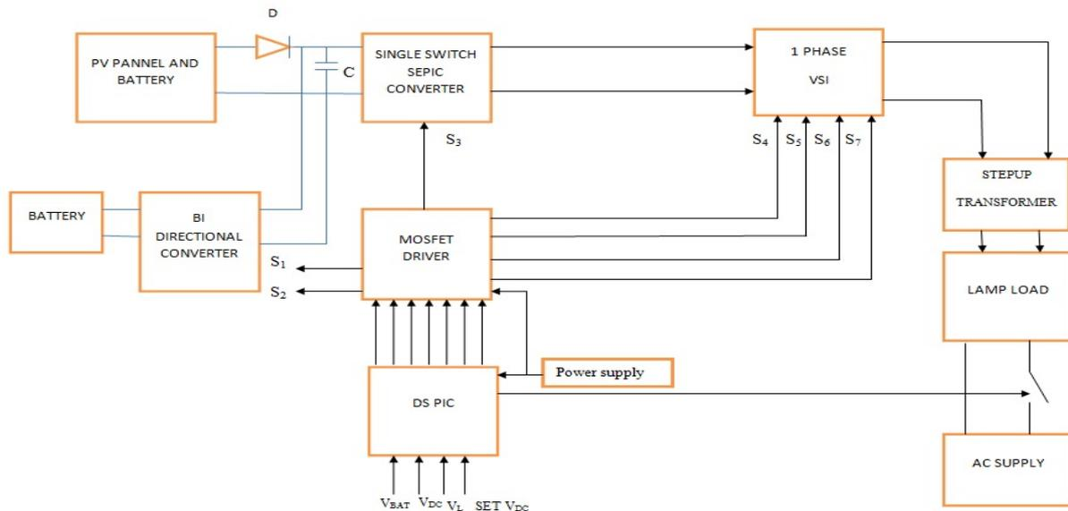
Fig1.1 Block Diagram for Proposed Converter
