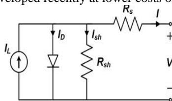
Although they are reduced in energy conversion efficiency from single crystalline "siwafers", they are also much easier to produce at comparably lower costs. PV arrays are built up with combined series/parallel combinations of PV solar cells, which are usually represented by a simplified equivalent circuit model such as shown in Figure. 1.2
