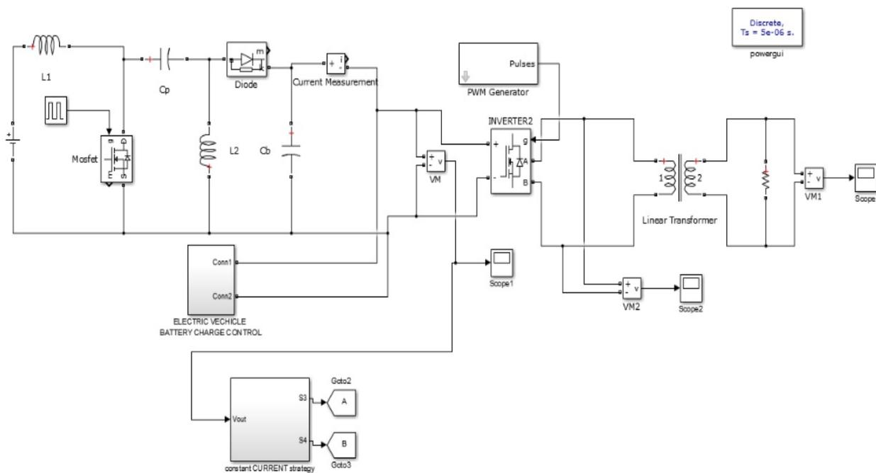
Fig.1.4 Circuit Diagram for Proposed Converter with Simulation
