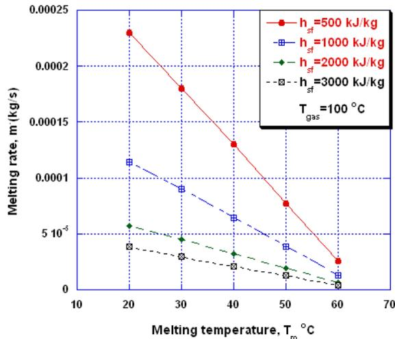
Fig. 3: Effect of melting temperature on melting rate at different  $h_{sf}$
