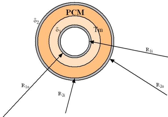
Fig. 1: Schematic representation of the domain under consideration.
