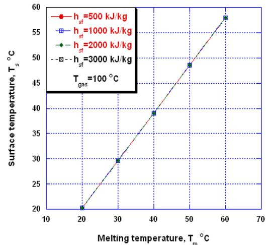
Fig. 4: Effect of melting temperature on surface temperature at different  $h_{sf}$
