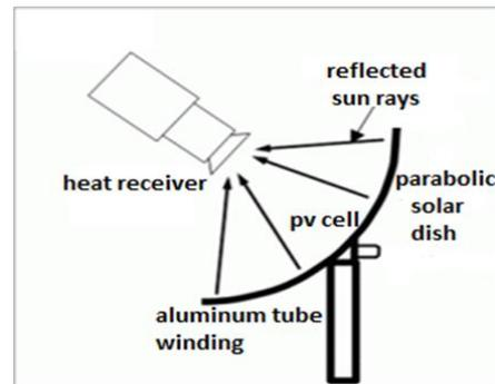
Fig 5 Parabolic solar dish collector
