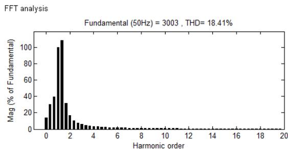
Fig 7: output wave form for Hybrid system and THD level
