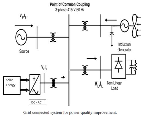
Fig.1 Single line diagram for Hybrid system
