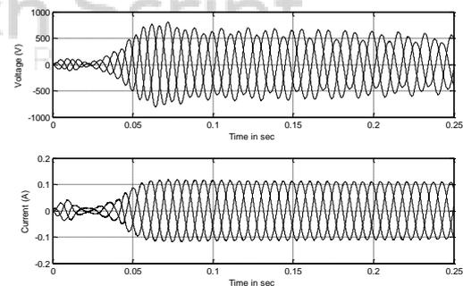
Fig 6: Input waveform without hybrid filter
