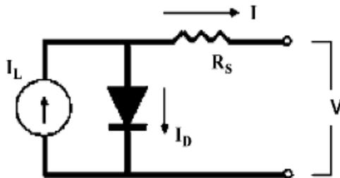
Fig 4.Solar-Cell Equivalent Circuit.
